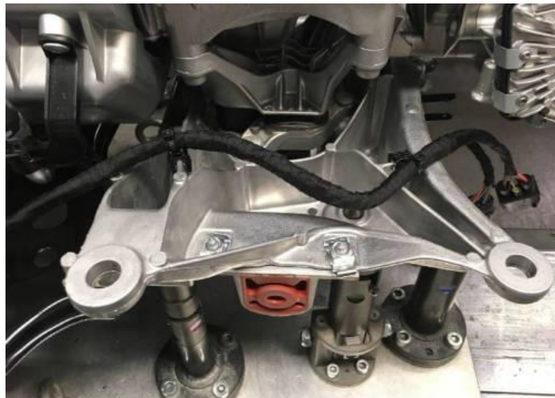
Figure 7. New routing and wrapping of the aft part of the transmission harness.
