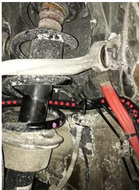
Figure 6. Routing the rubber hose.
