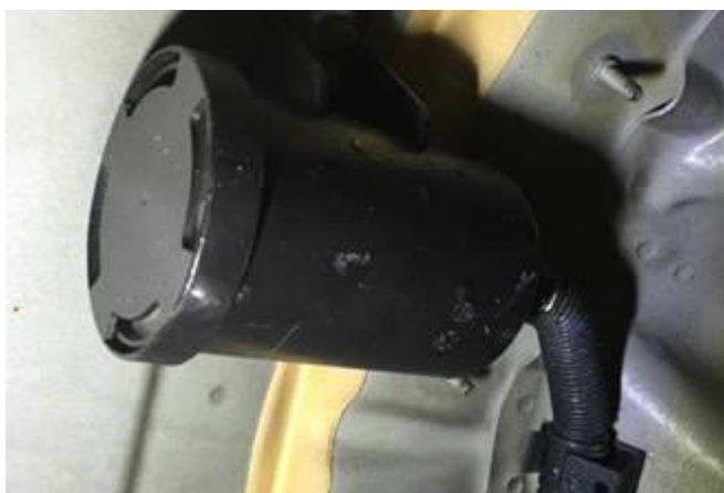
Figure 10. Remove original NVLD filter.
