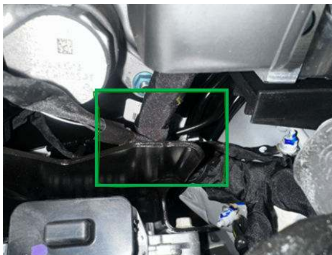
Fig. 2 Correctly Routed Harness
