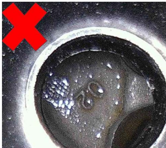
Fig. 4 Umbrella Valve Seal - Missing
