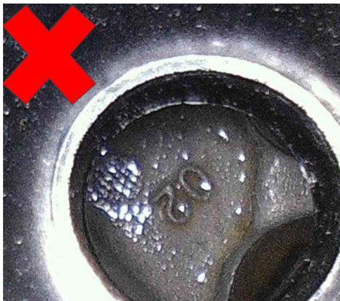
Fig. 5 Umbrella Valve Seal - Missing
