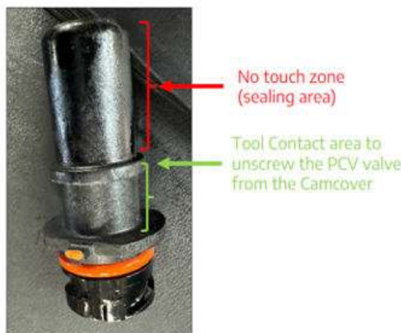
Fig. 2 PCV Valve During Removal
