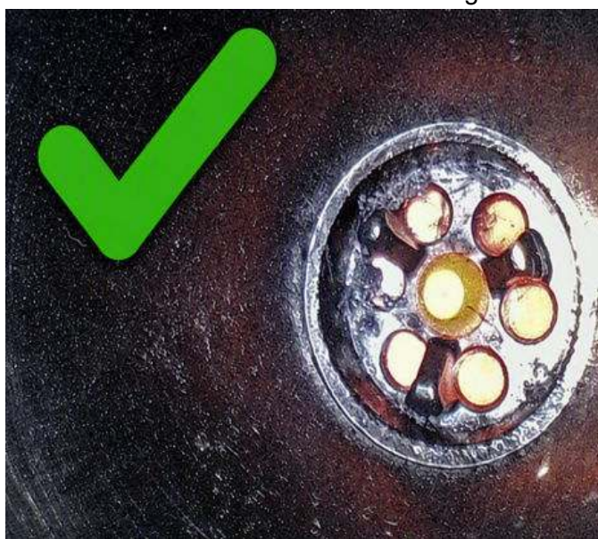
Fig. 6 Umbrella Valve Seal - Present
