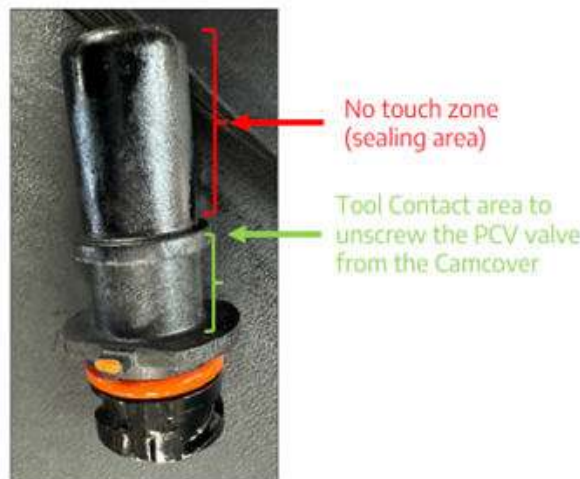
Fig. 2 PCV Valve During Removal
