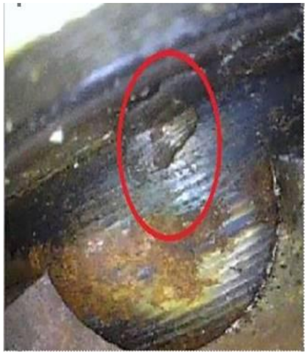
Figure 3: Metallic particles in the hub.
