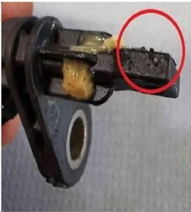
Figure 2: Metallic particles in the speed sensor.
