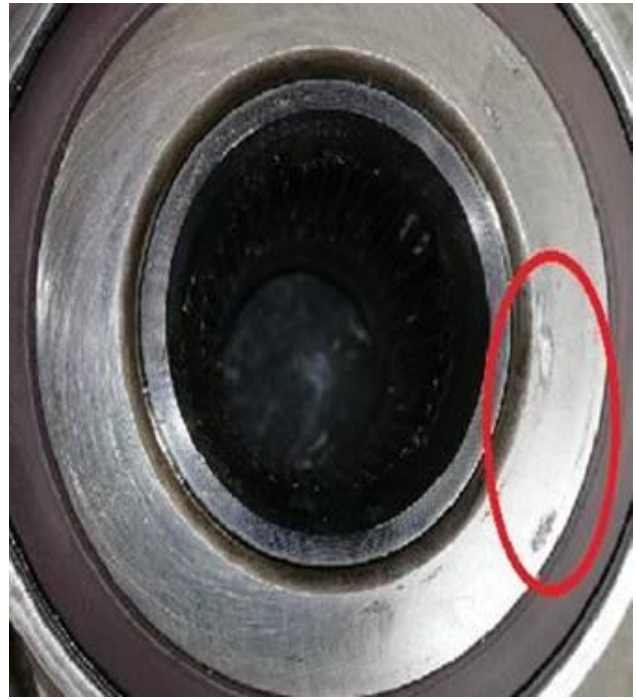
Figure 5: Metallic particles/damage in the wheel hub/bearing.
