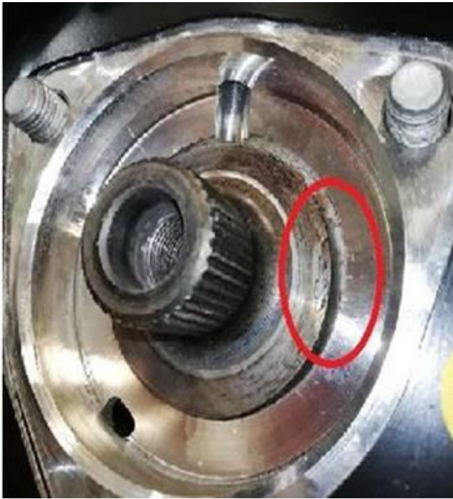
Figure 4: Metallic particles/damage in the wheel hub/bearing.
