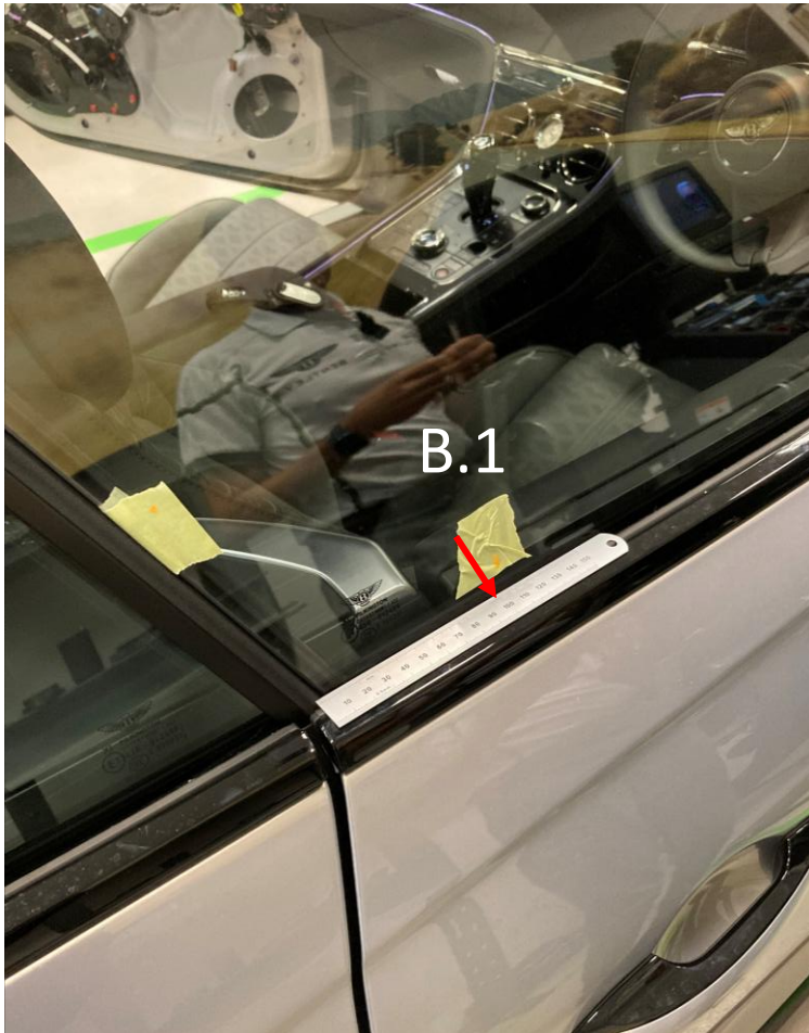
Mark on tape 100mm from div bar (B.1)
