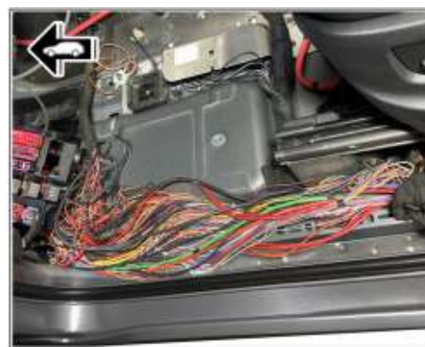
Exposed main wire harness in the passenger compartment, front left.
