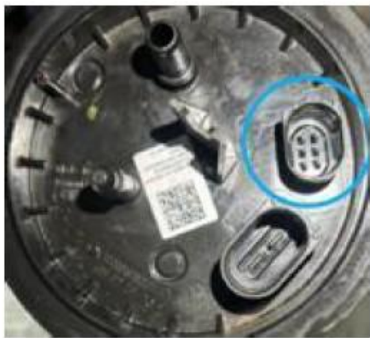
Figure 1. The 6-pin connector of the electric fuel pump is circled above in blue.
