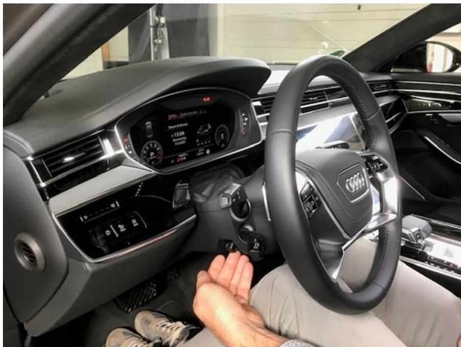
Figure 1. 40 kg force pushing steering wheel upward.
