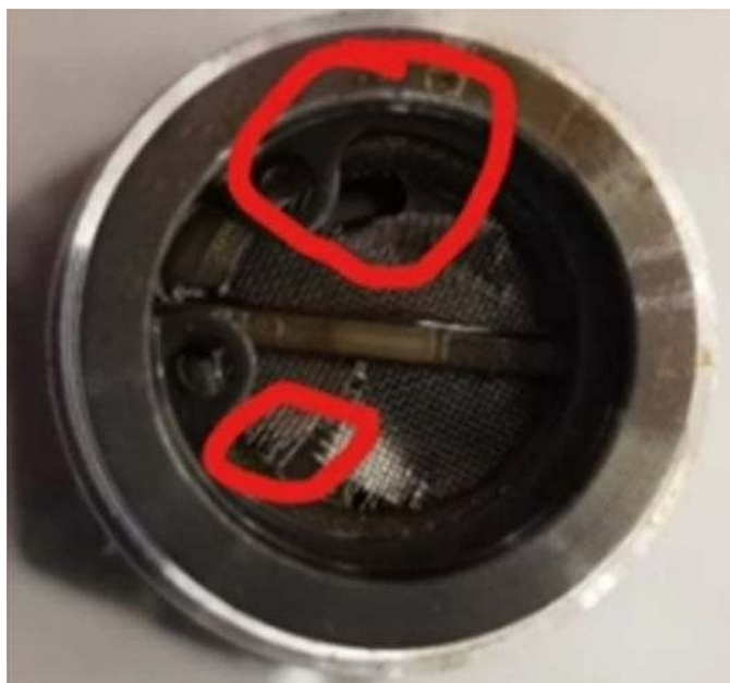
Fig. 2 OCV Filter Torn
