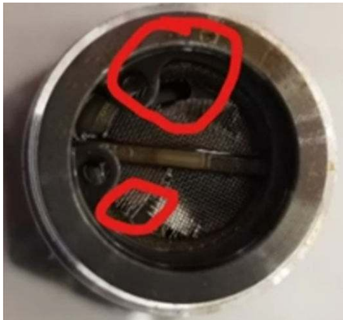
Fig. 2 OCV Filter Torn
