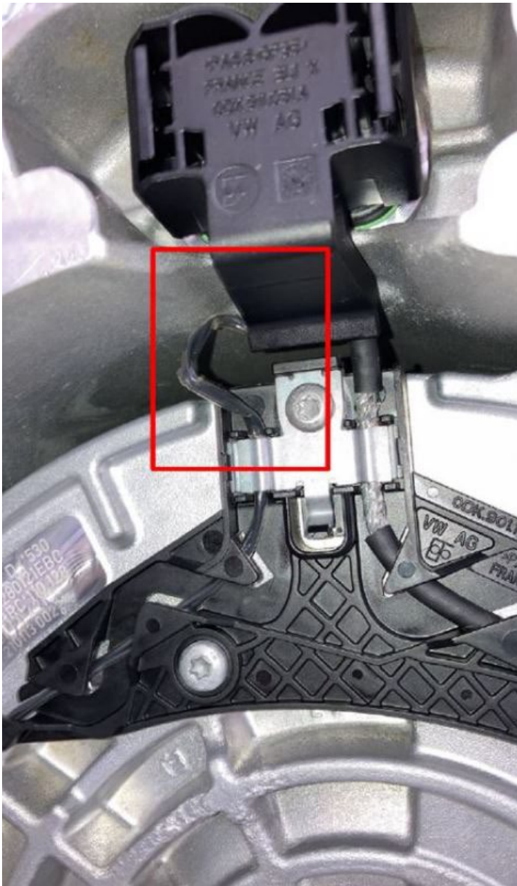
Figure 1. Wire not fitted correctly
