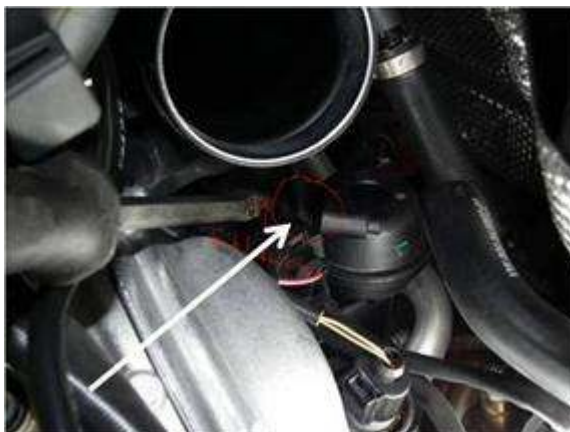
Figure 2. Vacuum hose not connected.
