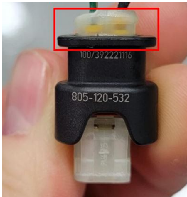
Fig. 3 Connector (D3157A) Not Fully Seated
