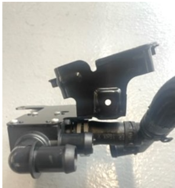
Fig. 1 Correct Hose #1 Location
