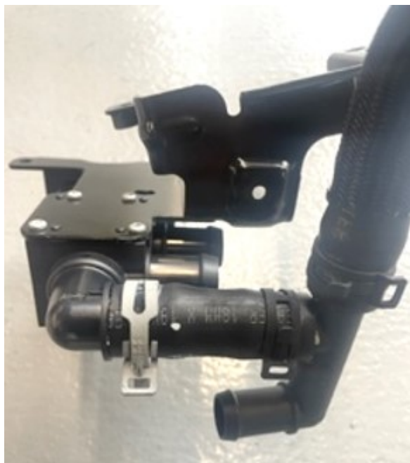
Fig. 2 Incorrect Hose #1 Location
