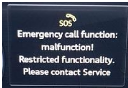
Figure 1. Emergency call malfunction warning.
