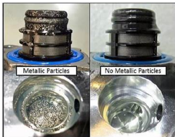
Figure 2. N290 Fuel Metering Valve and Valve Bore
