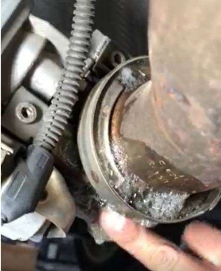
Figure 1. Example of exhaust leak at exhaust flap.
