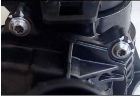
Marking Example 1: Draw marking lines over the screws and the thermostat cover as shown above.
