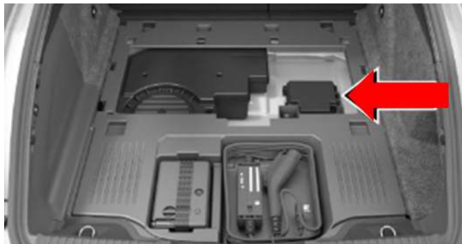
Fig. 2 Rear PDC Location
