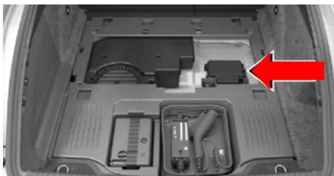
Fig. 2 Rear PDC Location
