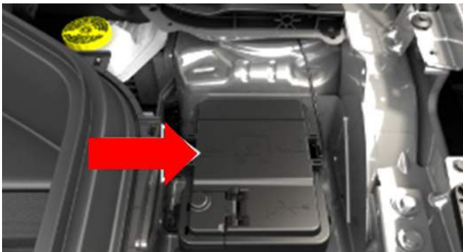
Fig. 2 Front PDC Cover
