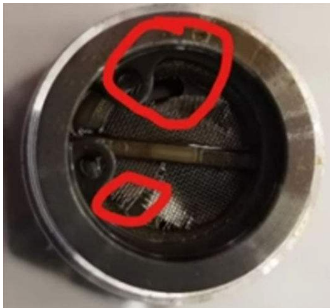
Fig. 2 OCV Filter Torn
