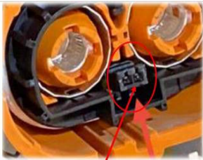
Broken interlock connector
