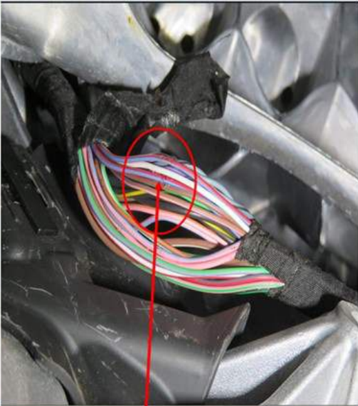
Wiring harness cut near rear e-ATS
