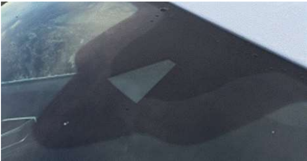
Figure 1. Viewing area fogged up from outside.
