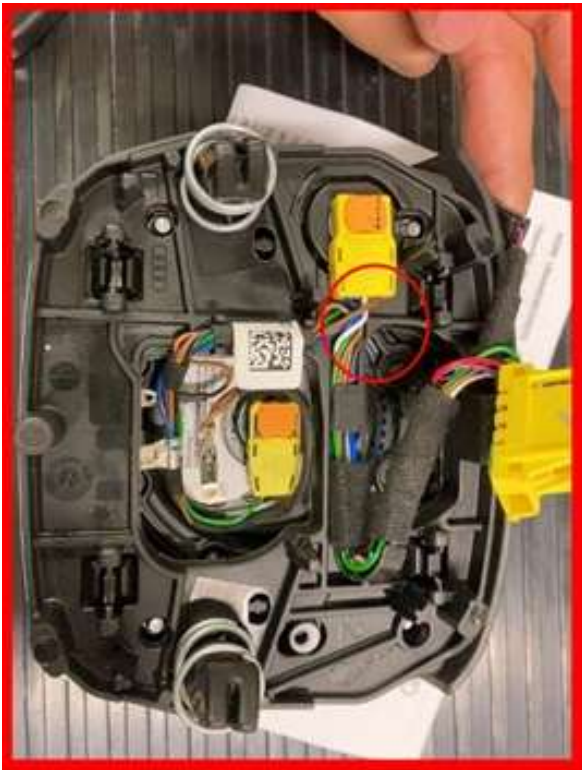
Figure 1. Check the routing of the wiring inside the driver airbag.
