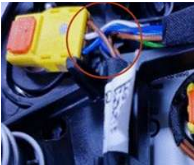
Figure 2. Check the routing of the wiring inside the driver airbag.
