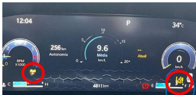
Fig. 1 Illuminated Collision Warning Light and Lane Keep Light On The IPC
