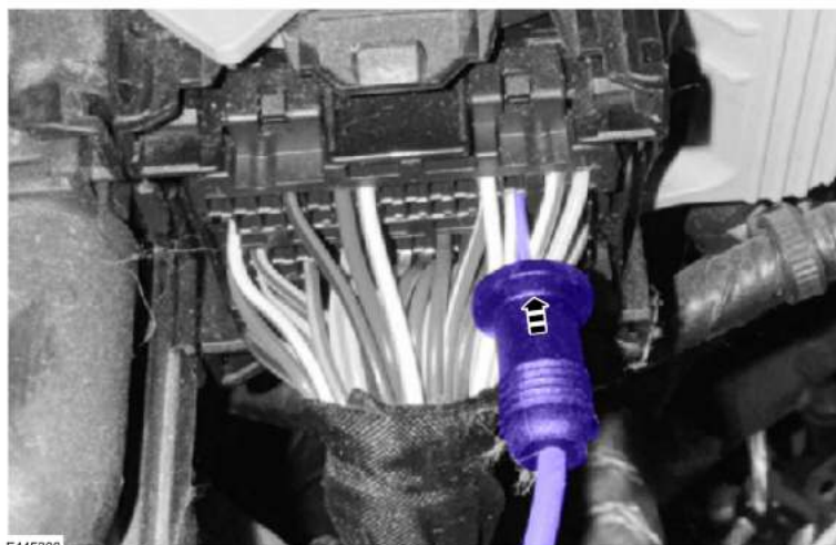
Figure 4 - Back probing a PCM connector shown, other connectors are similar
