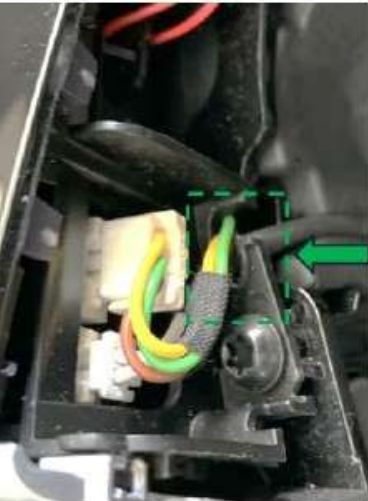
Figure 2. Correct wire routing on left side.
