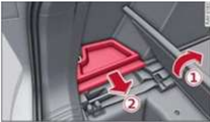
Figure 1: Fuse carrier installation location: luggage compartment on left, open cover.
