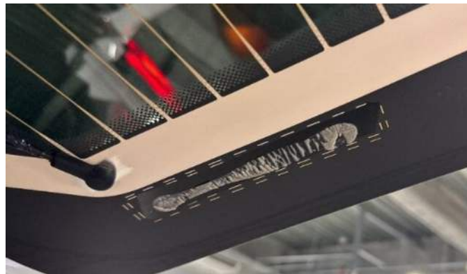
Fig. 5 Liftgate Damper Location - Missing Damper
