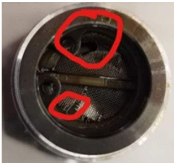
Fig. 2 OCV Filter Torn
