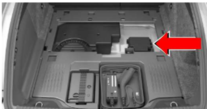
Fig. 1 Rear PDC Location
