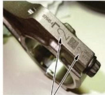
These are manufacturing marks, and do not indicate the cylinder number.
