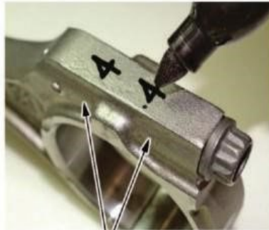
Mark the connecting rod and rod cap with the cylinder number.
