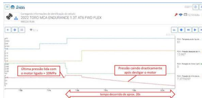
Fig. 1 Leak Test - KO Result
