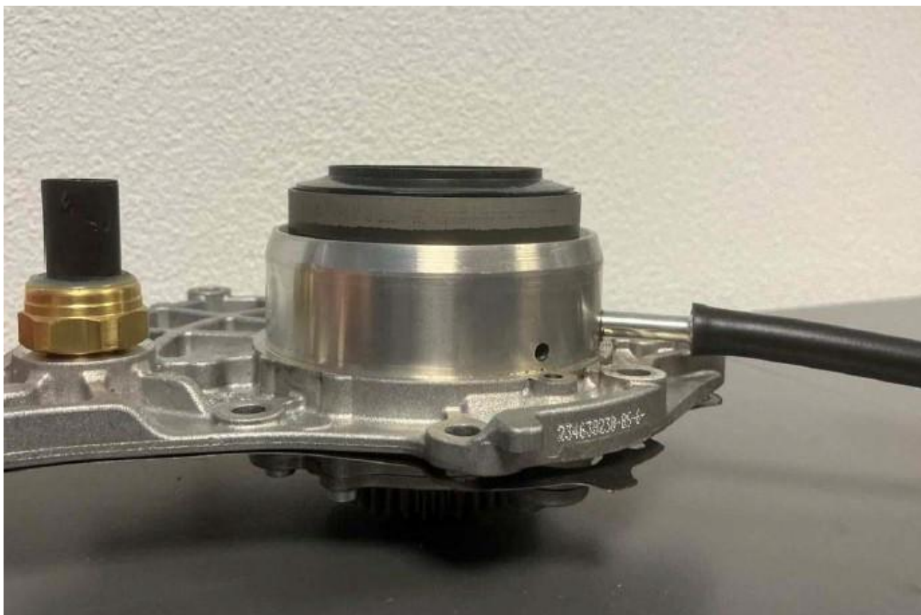
Figure 4. Modulating piston correctly deployed (end position, actuated)
