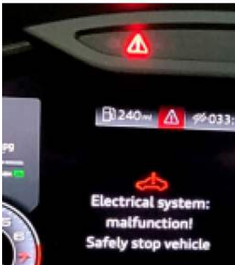
Figure 1. Warning lamp associated with message.
