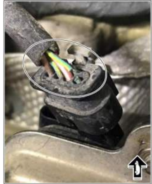
Electric wiring harness for exhaust flap actuator
