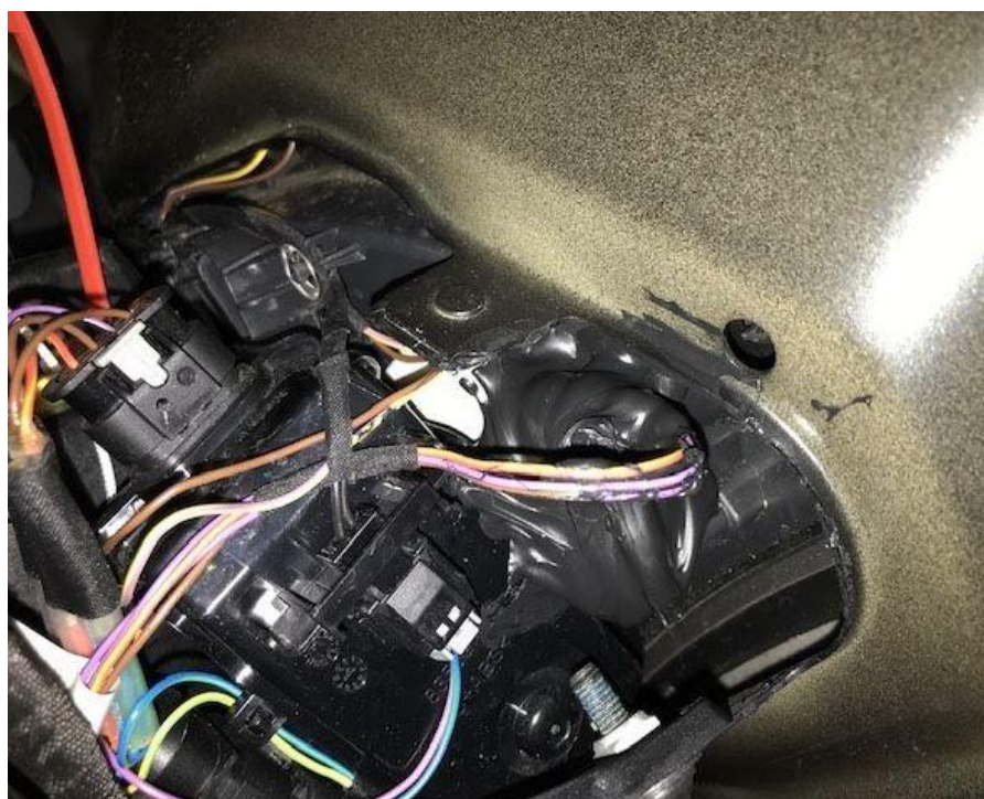
Figure 25: The entire connector and the connector point of the charging indicator must be covered with adhesive sealant.
