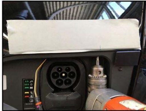
Figure 12: Use an angled drill/angle bit to drill to a depth of 15mm at the marked location.
