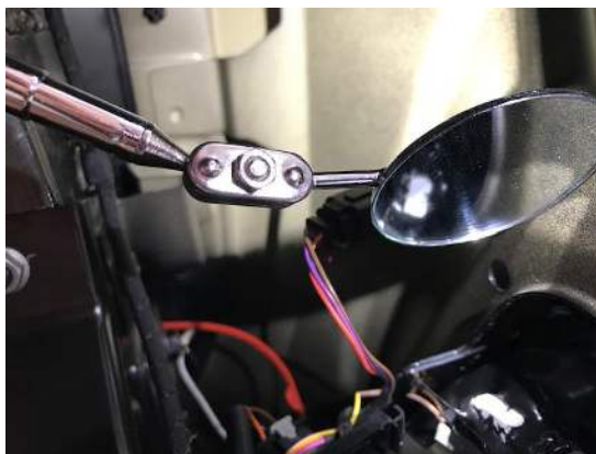
Figure 6: Use inspection mirror to carefully examine the charging indicator connector.
