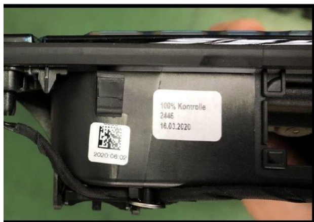
Figure 8: The charging indicator connector pictured is the updated part.
