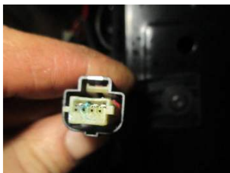
Figure 3: Evidence of water intrusion in the connector housing.
