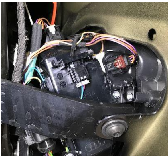
Figure 24: The connector should be completely surrounded by the adhesive sealant.
