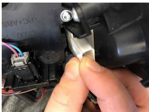
Figure 1: Crack in the connector point of the charging indicator.
