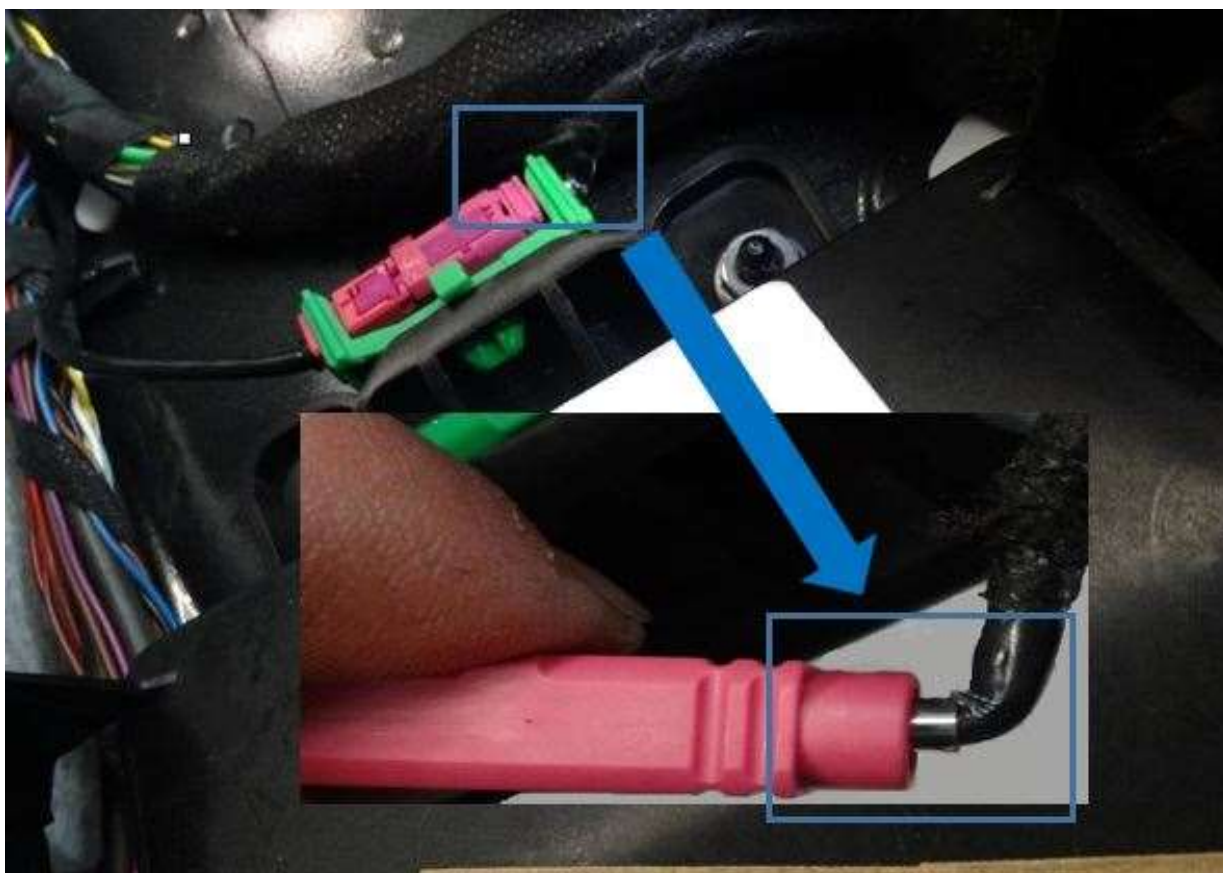
Figure 3. Loose plug on connector T2dx (see blue frame).
