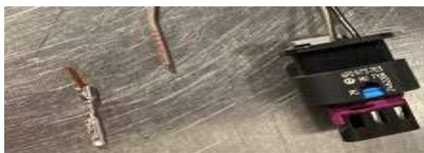
Figure 2: Wire damaged inside G31 connector
